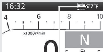
Air temperature gauge
