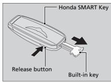
**2.** Slightly insert the built-in key from the opposite side into the key hole.
