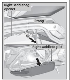
**5.** Install the right saddlebag opener onto the prong before closing the saddlebags.
