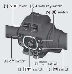
[1] **VOL** (volume control) lever: Push the lever up to increase the volume.
