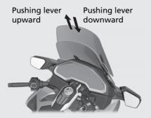
Turning the ignition switch to OFF will automatically lower the windscreen to its original position.
