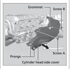
The right and left cylinder head side cover can be removed in the same way.
