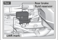
If the brake fluid level in either reservoir is below the LWR mark or the brake lever and pedal freeplay becomes excessive, inspect the brake pads for wear. If the brake pads are not worn, you most likely have a leak. Have your vehicle inspected by your dealer.
