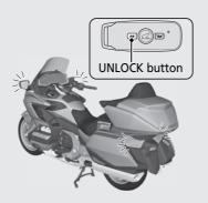
If you press the UNLOCK button, but nobody opens any of the compartments within about 30 seconds or about 30 seconds have passed after an opened compartment is closed, the compartments automatically will relock (Turn signals blink once).
