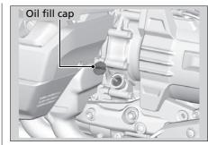
2. Securely reinstall the oil fill cap.
