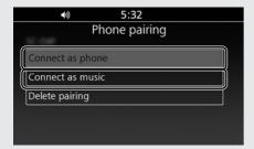
[Rider HS pairing] / [Passenger HS pairing] Select [Connect], and then press 👶 or ENT switch.
