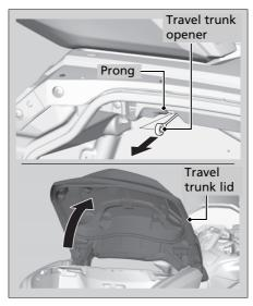
**3.** Install the travel trunk opener onto the prong before closing the right saddlebag.
