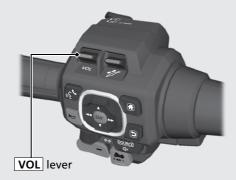
To mute the volume: Press and hold  $\frac{\text{SOURCE}}{\text{ID}}$  switch.
