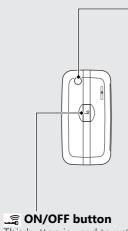
This button is used to activate or deactivate the Honda SMART Key system and also to confirm the activation status. P.99
