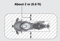
Anyone can operate the ignition switch and start the engine if your Honda SMART Key is within operating range of your vehicle, even if you are on the other side of a wall or window. If you are away from your vehicle but your Honda SMART Key is still within the system's operating range, switch the Honda SMART Key system to inactive.
