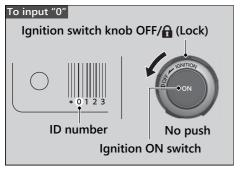
To input "1", push the ignition ON switch once, and then turn the ignition switch knob OFF/n (Lock) counterclockwise to input the next digit.
