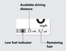
After refueling more than the reserve amount, the display returns to normal when the electrical system has been on for about a minute.
