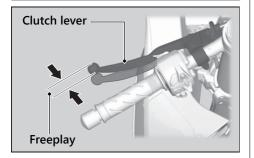
Check the clutch cable for kinks or signs of wear. If necessary, have it replaced by your dealer.
