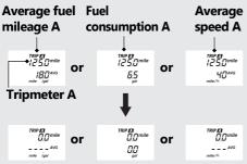
To reset the tripmeter B, average fuel mileage B, fuel consumption B, and average speed B (these are based on tripmeter B) together, press and hold the **SEL** button while tripmeter B is displayed.
