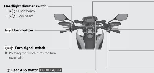
Switches the ABS function on the rear wheel on/off.
