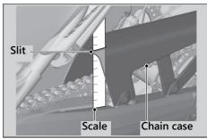
**4.** Pull up the drive chain and check the slack between the top of the swingarm and the drive chain by the scale.
