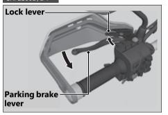
Place your vehicle on a firm, level surface. Stop the engine and push your vehicle while set the parking brake to check the efficacy of the parking brake.
