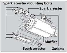
**4.** Use a brush to remove carbon deposits from the spark arrester screen. Be careful to avoid damaging the spark arrester screen. The spark arrester must be free of breaks and holes. Replace, if necessary. Check the gasket. Replace, if necessary.
