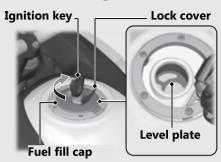
Do not fill with fuel above the level plate. Fuel type: Unleaded gasoline only
