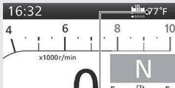
Air temperature gauge
