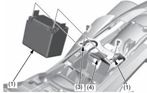
(1) battery (3) negative (-) terminal bolt (2) positive (+) terminal bolt (4) battery band
