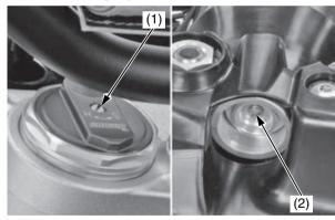
(1) compression damping adjuster(2) rebound damping adjuster
