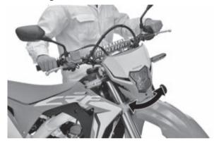
2. Stand in front of your motorcycle, grab the fork (at the axle), look at the steering head, and push the fork in and out (toward the engine) to check for play in the steering head bearings.
