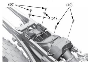
(49) air cleaner housing mounting A bolts (50) air cleaner housing mounting B bolts
