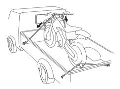
To secure your motorcycle, brace the front wheel against the front of the truck bed or trailer rail. Attach the lower ends of two straps to the tie-down hooks on truck bed or trailer rail. Attach the upper ends of the straps to the handlebar (one on the right side, the other on the left), close to the fork.
