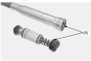
(5) fork bolt and fork damper assembly threads
