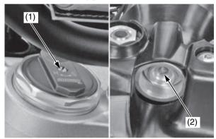
(1) compression damping adjuster(2) rebound damping adjuster
