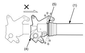
(1) outer tube (4) axle holder (5) fork dust seal
