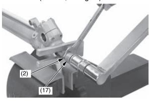
(2) fork center bolt lock nut (17) fork center bolt
