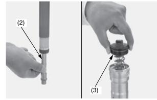
(2) fork damper piston rod (3) fork bolt assembly
