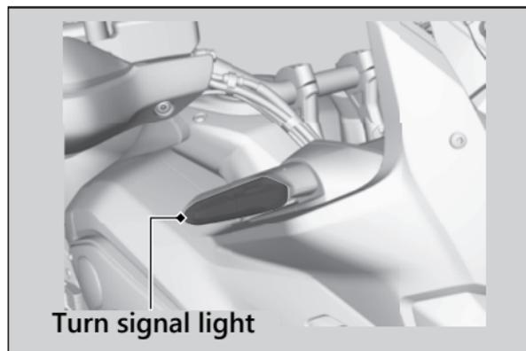
The front and rear turn signal lights use several LEDs.
