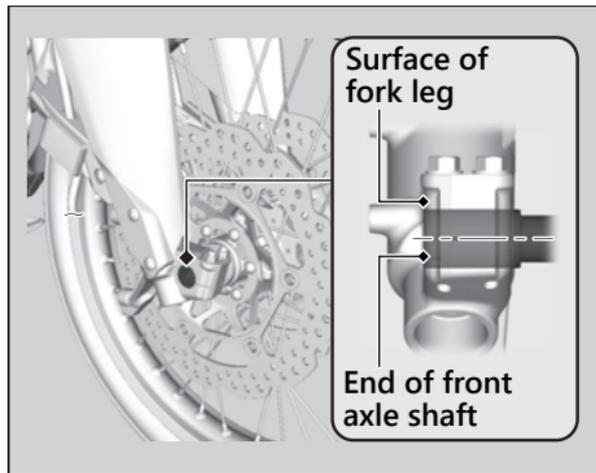
4. Tighten the right axle pinch bolts to hold the axle.
