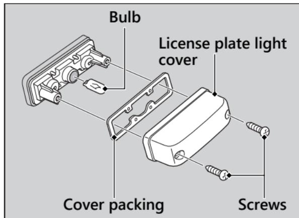
4. Install a new bulb and parts in the reverse order of removal.
