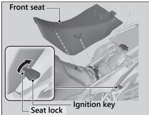
1. Insert the ignition key into the seat lock, and turn and hold the key clockwise to unlock the front seat.
