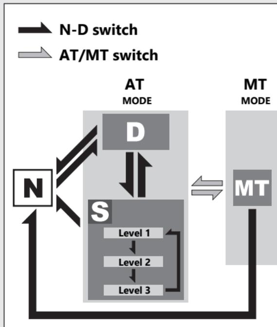
**Neutral (N):** Neutral is selected automatically when you turn the ignition switch to the ON position.
