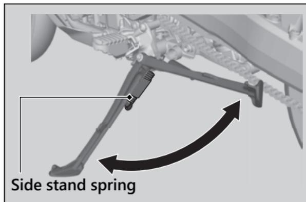
1. Check that the side stand operates smoothly. If the side stand is stiff or squeaky, clean the pivot area and lubricate the pivot bolt with clean grease.
