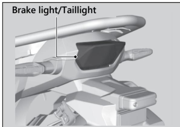
The brake light and taillight uses several LEDs.
