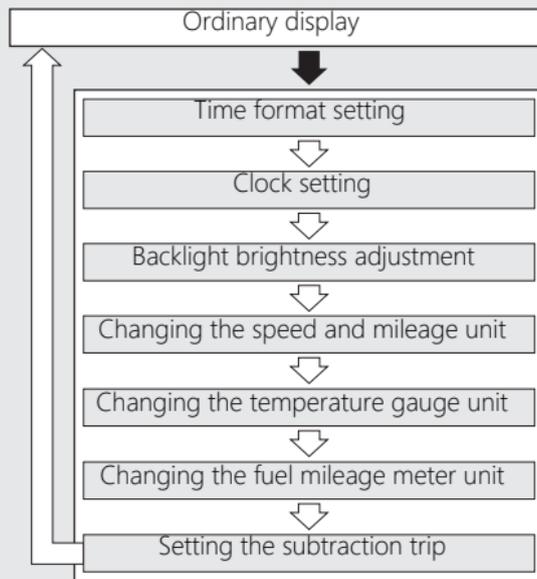
If the ignition switch is turned to the OFF position or none of the **MODE**, **SEL** ▲ (up), **SEL** ▼ (down), buttons is pressed for about 30 seconds, the control is automatically switched from the setting mode to the ordinary display.
