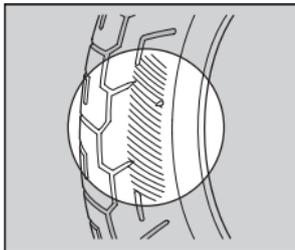
Inspect the tires for signs of abnormal wear on the contact surface.
