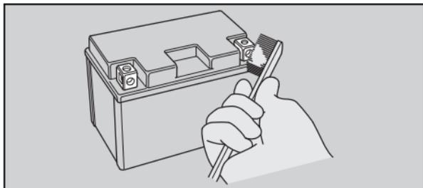
4. After cleaning, reinstall the battery. The battery has a limited life span. Consult your dealer about when you should replace the battery. Always replace the battery with another lithium-ion (li-ion) battery of the same type.
