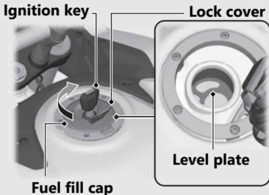
Do not fill with fuel above the level plate.
