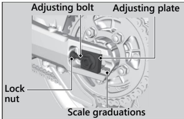
5. Turn both adjusting bolts an equal number of turns until the correct drive chain slack is obtained. Turn the adjusting bolts counterclockwise to tighten the chain. Turn the adjusting bolts clockwise and push the rear wheel toward the front to provide more slack. Adjust the slack at a point midway between the drive sprocket and the driven sprocket. Check the drive chain slack. ► P. 129
