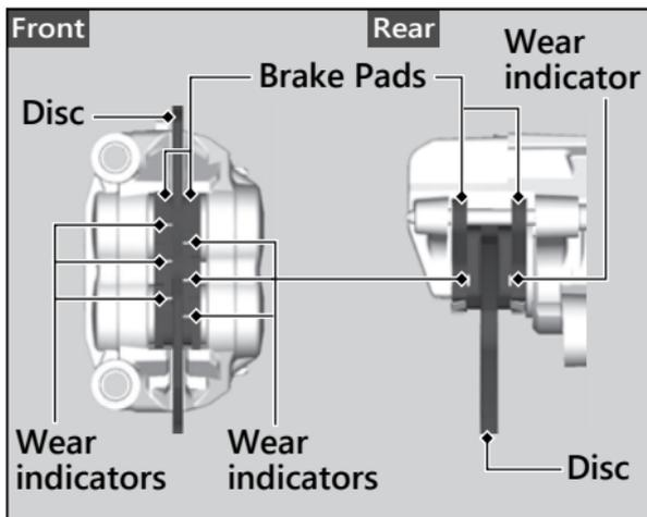
1. **Front** Inspect the brake pads from in front of the brake caliper.
