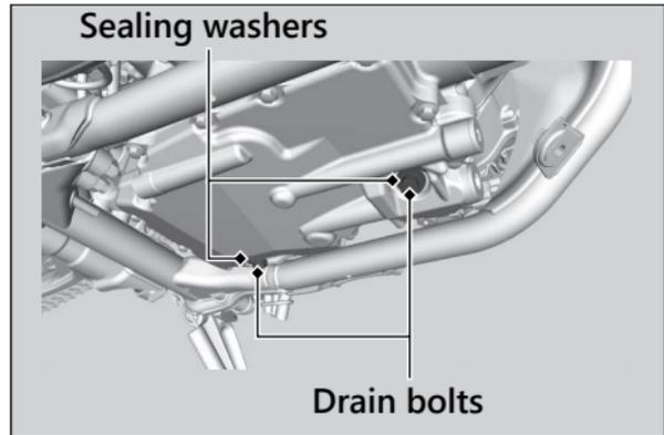
6. Remove the oil fill cap, drain bolts, and sealing washers to drain the oil.
