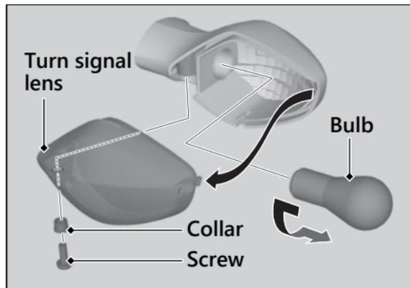
4. Install a new bulb and parts in the reverse order of removal.
