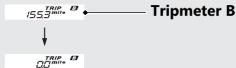
Also, the tripmeter A, average fuel mileage, and fuel consumption will automatically reset by refueling more than the reserve amount and riding your motorcycle for 0.06 mile (0.1 km).
