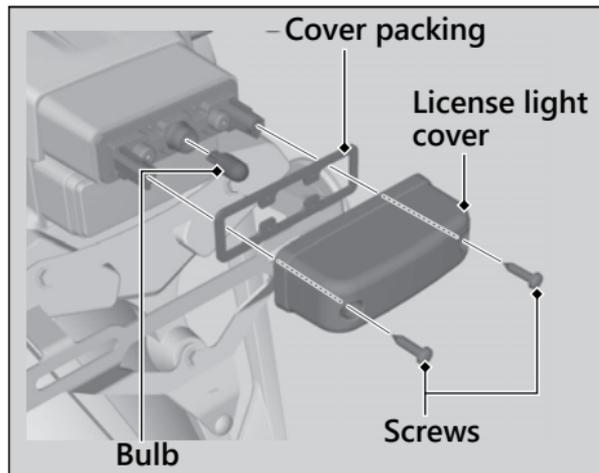
3. Install a new bulb and parts in the reverse order of removal.
