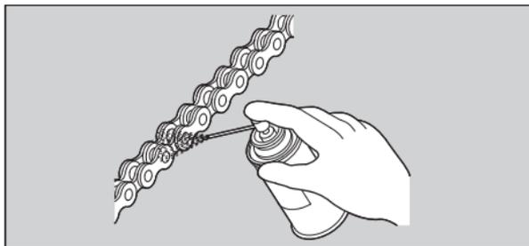
Do not use a steam cleaner, a high pressure cleaner, a wire brush, volatile solvent such as gasoline and benzene, abrasive cleaner, chain cleaner or lubricant NOT designed specifically for O-ring chains as these can damage the rubber O-ring seals.
