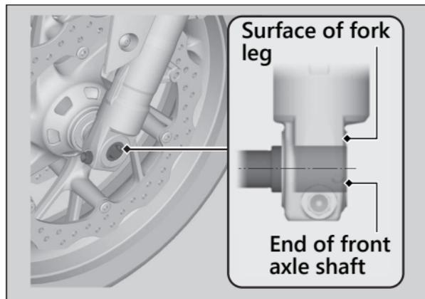
4. Tighten the left axle pinch bolt to hold the axle.
