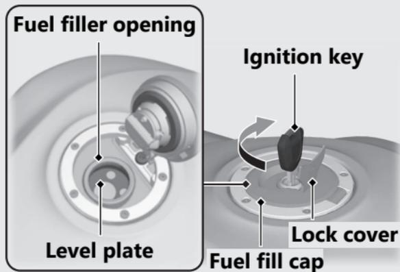
Do not fill with fuel above the level plate.
