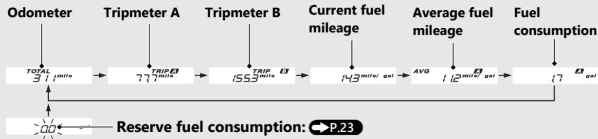
The average fuel mileage and fuel consumption will be based on tripmeter A.
