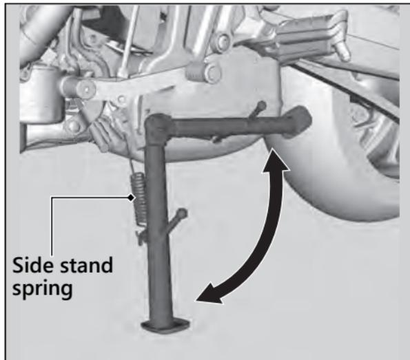
1. Check that the side stand operates smoothly. If the side stand is stiff or squeaky, clean the pivot area and lubricate the pivot bolt with clean grease.
