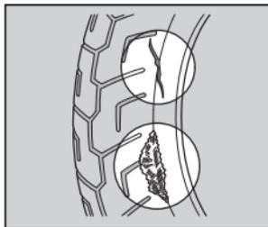
Inspect the tires for cuts, slits, or cracks that exposes fabric or cords, or nails or other foreign objects embedded in the side of the tire or the tread.
