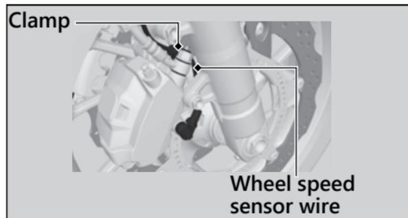
9. Install the right brake caliper and tighten new mounting bolts.
