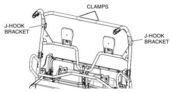
11. Secure the sides of the upper panel to the J-hook brackets using two 6 x 25 mm screws, flat washers and tie-down rings as shown. Leave the hardware loose for now.
