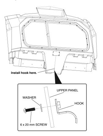
7. Place the upper panel on the outside of the frame. Align the upper panel with the lower panel by sliding the slots from the upper panel over the lower panel as shown. (The cargo bed must be halfway between open and closed.)
