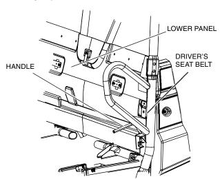
4. Re-install the seat back cushions over the lower panel using four of the screws removed in Step 2 as shown.
