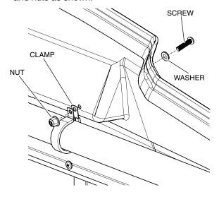
15. Lower the cargo bed. Using the lower panel as a template, drill six holes into the upper panel using a 5/16 inch drill bit.
