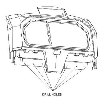
16. Fasten the lower and upper panels together at the locations drilled in Step 10 using six trim clips.
