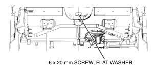
6. Install the hook onto the smooth side of the upper panel using a 6 x 20 mm screw and flat washer as shown.
