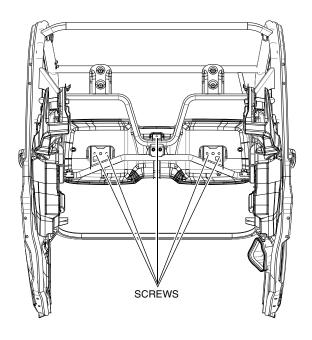
3. Align the lower panel in place (textured side facing rearward) with the inside of the frame, where the seat cushion was removed.
