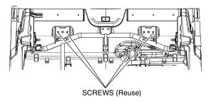
5. Install a 6 x 20 mm screw and flat washer into the middle hole location as shown.
