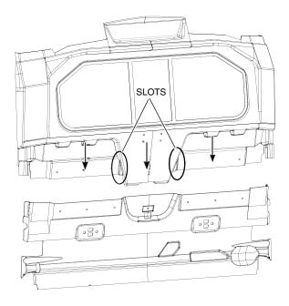
8. Ensure the hook on the upper panel secures onto the frame as shown.
