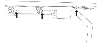
16. Run the Audio Extension Cable to the A pillar and down to the dash. Zip tie as needed.
