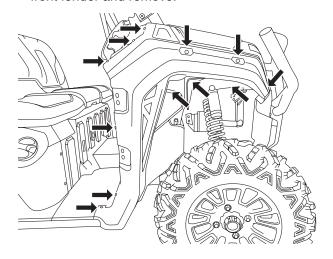
4. Undo any accessories that are blocking access to driver and passenger rear down-tube. Roll up the rear window netting and secure out of the way.
