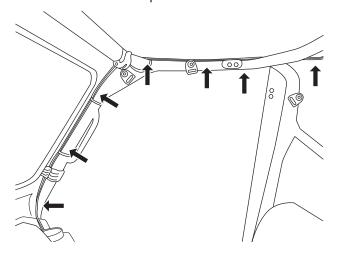
17. Run the cable between the dash and the A pillar into the fender cavity.
