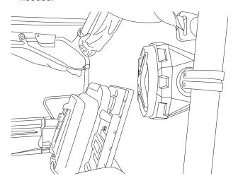
11. Secure the cage pod in its final location by tightening the two (2) M6 hex head bolts on the swivel adapter mount from Step 6 with an 8 mm wrench.
