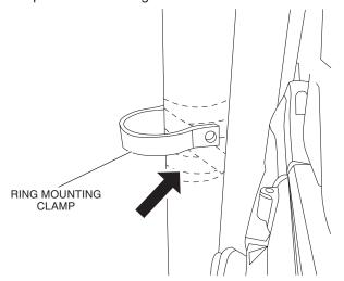
8. Place the cage mount pod in its final mounting location and secure to the clamps using the two (2) M6 Allen head bolts and washers with a 5 mm Allen wrench.
