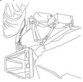
13. Run the cable across the rear roof bar. Run under the Velcro straps of the soft top if equipped and zip tie to the cage in marked location. If equipped with a roof, route cables around any roof clamps and zip tie as needed.
