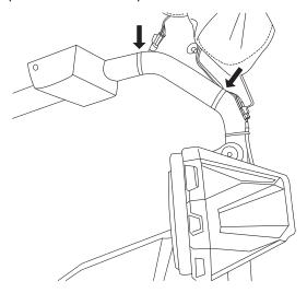
15. Plug in the Audio Extension Cable into the Rear Speaker Harness. Run along the passenger side roof bar and zip tie in the marked locations. If equipped, run the harness under all soft top straps.
