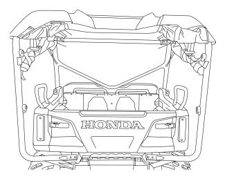
5. Install four (4) Set Screws into each speaker pod in the locations shown.
