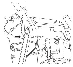
18. Run the Audio Extension Cable into the under-hood cavity and connect to the Rear Speaker Output of the radio MCU. Bundle and zip tie any excess length in the fender cavity.
