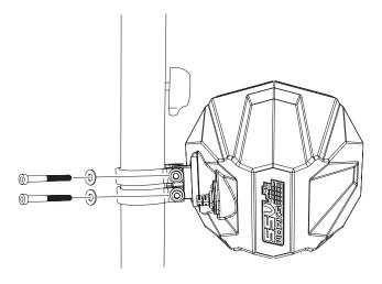
Adjust the speaker so the center of the ring clamps is 4" below the window net mounting bolt and the speaker pod. Aim the speaker towards the center of the front roof crossbar.
