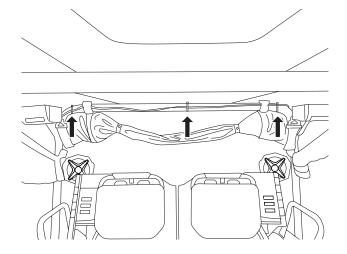
14. Run passenger leg of the speaker harness over the rear roof cross bar and plug into the cage pod's two-pin connector and zip tie in the marked locations.
