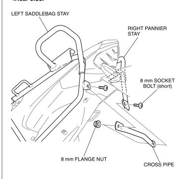
12. Tighten all loosely installed hardware to the specifications in the torque chart.
