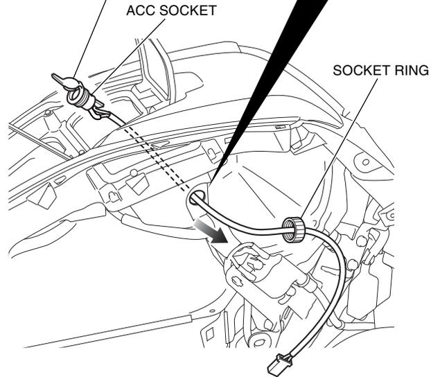
8. Remove the dummy connector 6P connector as shown.
