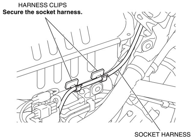
23. Secure the socket harness with the wire tie as shown.
