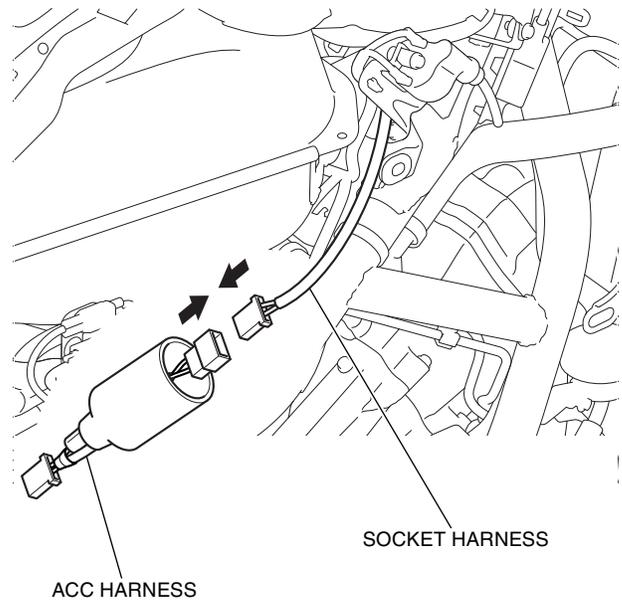
14. Cover the connector with the harness boot as shown.
