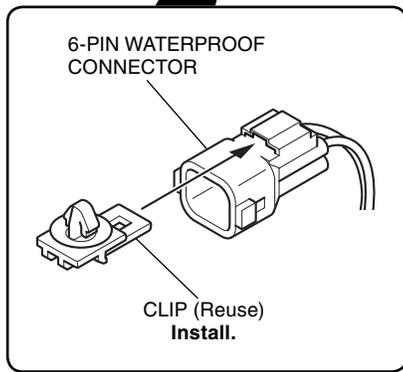
10. Install the 6-pin waterproof connector as shown.
