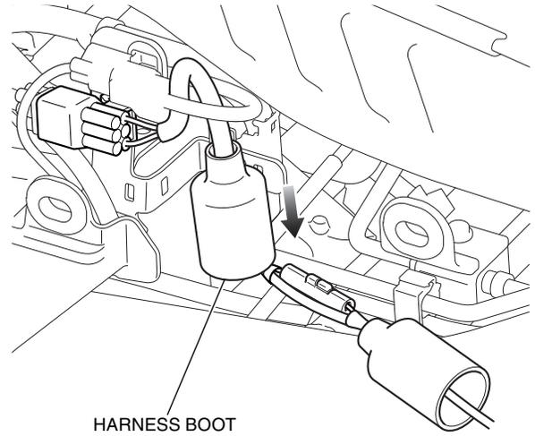
17. Secure the sub harness with the wire tie as shown.
