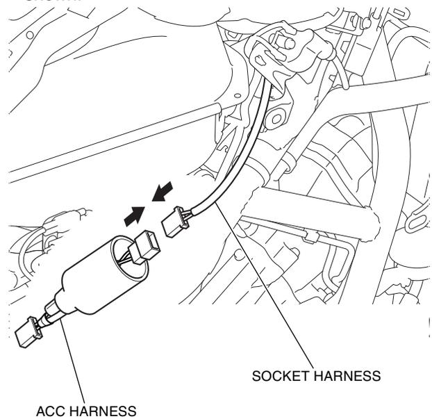
17. Cover the connector with the harness boot as shown.
