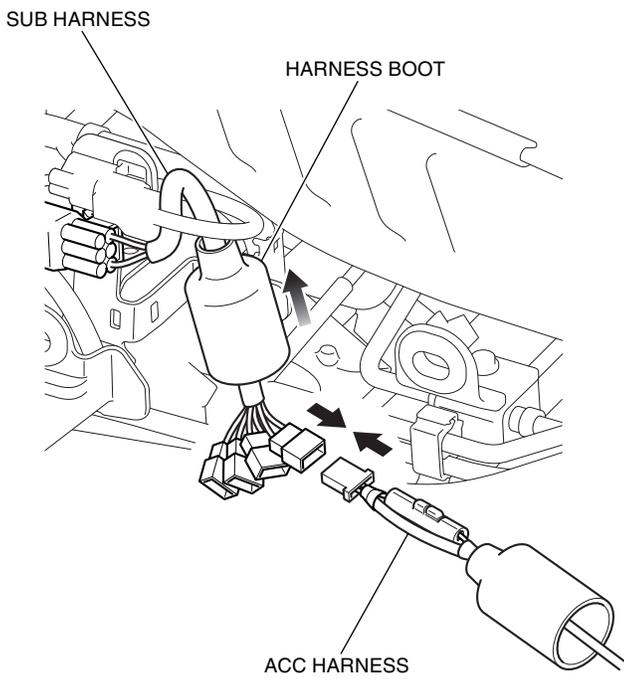
16. Cover the connectors with the harness boot as shown.
