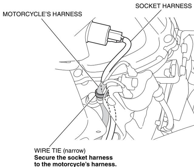
24. Secure the ACC harness with the wire tie as shown.
