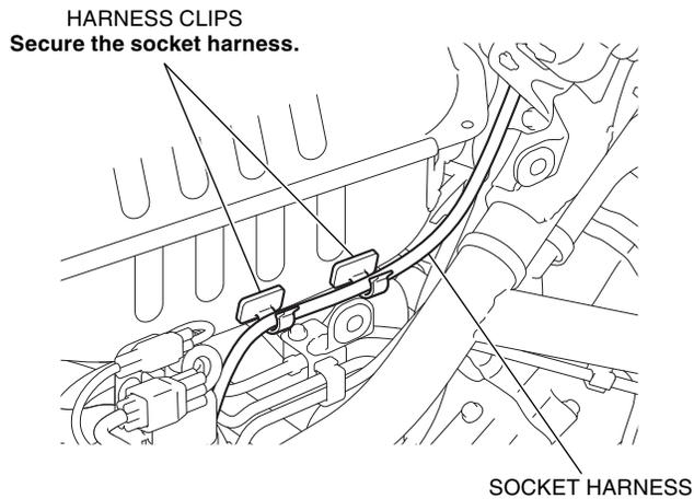
20. Secure the socket harness with the wire tie as shown.
