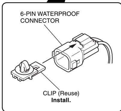
13. Install the 6-pin waterproof connector as shown.
