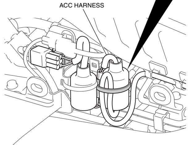
22. Attach the safety label in the position shown.
