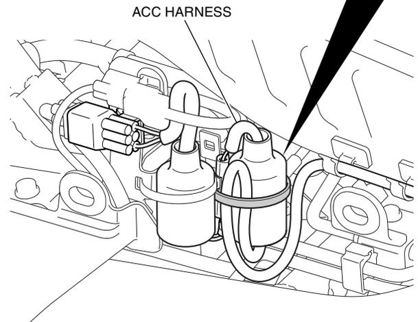
25. Attach the safety label in the position shown.
