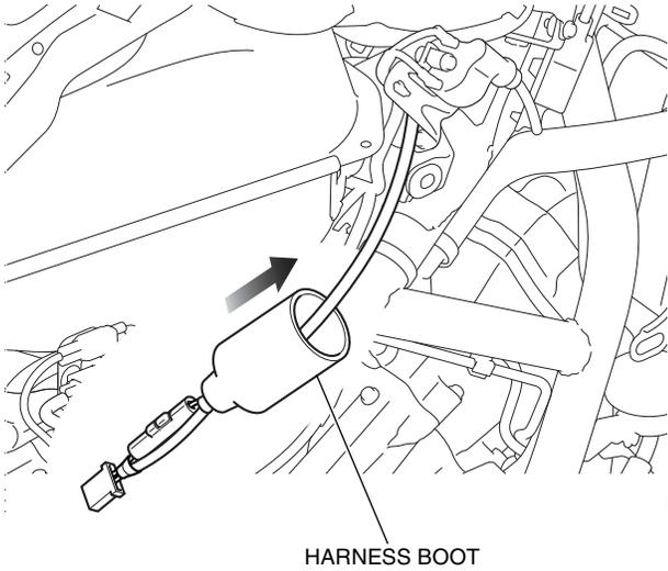
15. Connect the ACC harness to the sub harness as shown.
