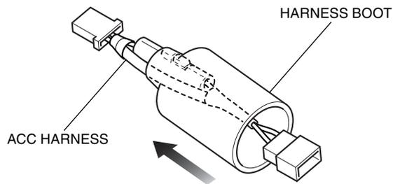
16. Connect the ACC harness to the socket harness as shown.
