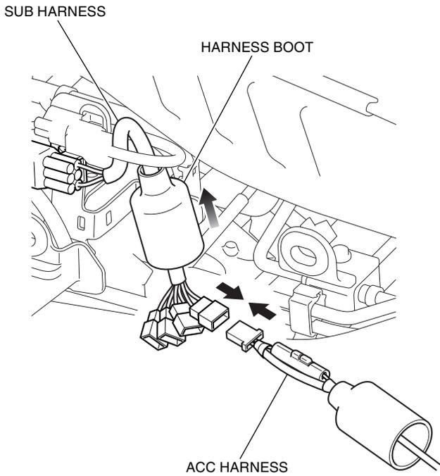
19. Cover the connectors with the harness boot as shown.
