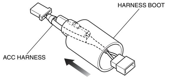
13. Connect the ACC harness to the socket harness as shown.
