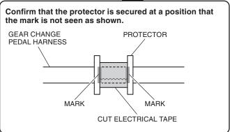
10. Secure the gear change pedal harness with the wire tie as shown.
