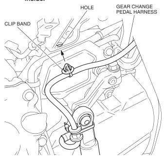
19. Secure the gear change switch harness with the wire tie as shown.
