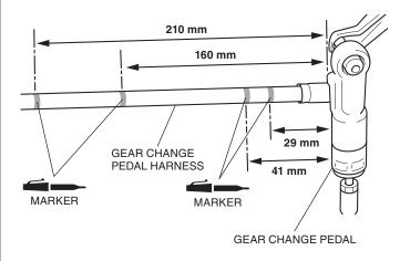
6. Cut a piece of electrical tape as shown to the indicated dimension.
