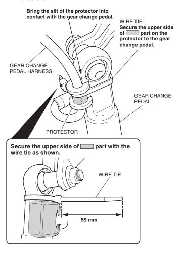
11. Secure the gear change pedal harness in the position of the dimension shown.
