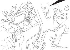
5. Mark the gear change pedal harness at the position of the dimensions shown.
