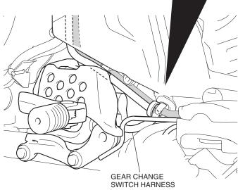
23. Route and connect the gear change switch harness as shown.
