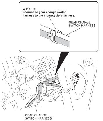
25. Secure the gear change switch harness with the wire tie as shown.
