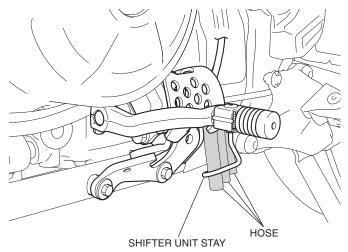
21. Route the gear change switch harness as shown.
