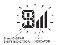
The S gear shift indicator, level indicator and D gear shift indicator blink alternately 5 seconds after deregistration is completed.
