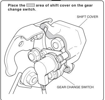
17. Install the gear change pedal as shown.
