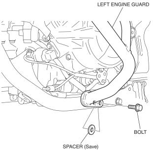
7. Remove the bracket as shown.
