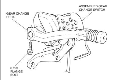
19. Install the assembled gear change switch as shown.
