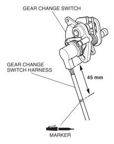
13. Loosely install the shifter unit stay to the gear change switch as shown.
