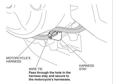
12. Mark the gear change switch harness in the position shown.
