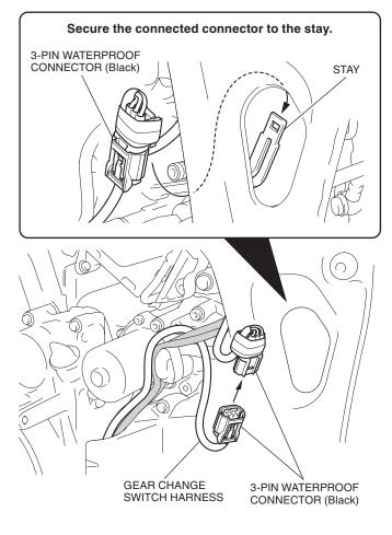
24. Secure the gear change switch harness with the wire tie as shown.
