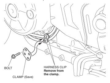
9. Remove the harness clips as shown.
