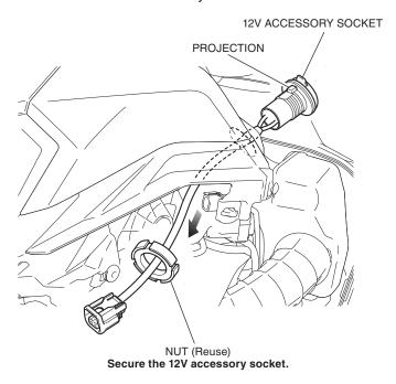
10. Connect the 12V accessory socket harness as shown.
