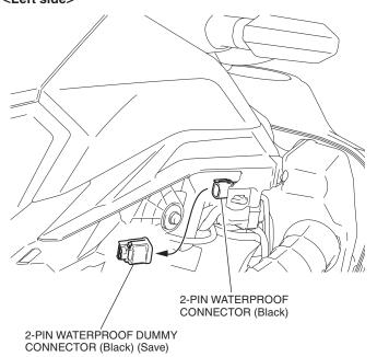
9. Install the 12V accessory socket as shown.
