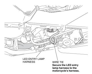
35. Route and connect the LED entry lamp harness as shown.
