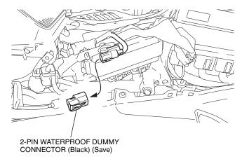
31. Remove the dummy connector as shown.
