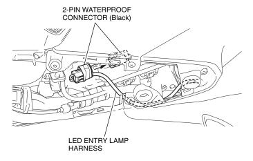
34. Secure the LED entry lamp harness with the wire tie.
