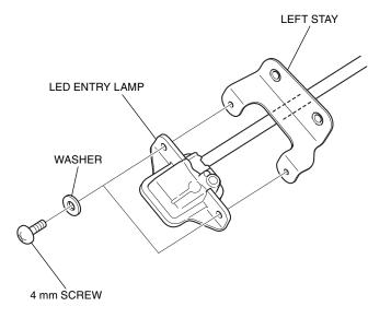
27. Route the LED entry lamp harness as shown and install the left stay.
