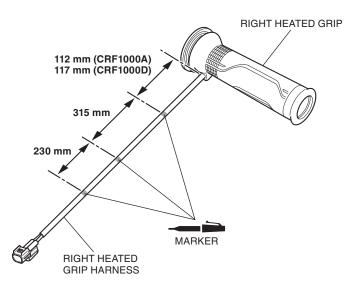
51. Install the clip bands at the marked positions as shown.
