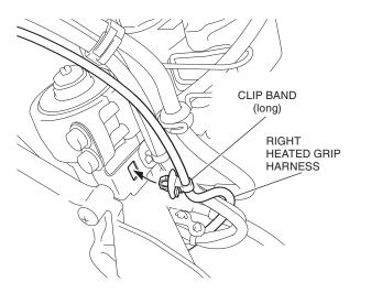
62. Secure the right heated grip harness with the clamps as shown.
