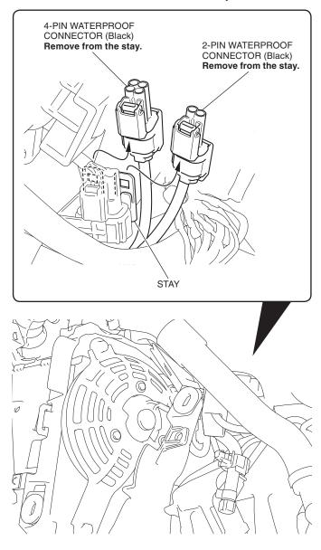
40. Remove the dummy connectors as shown.
