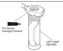
29. Apply the Pro Honda Handgrip Cement to the left handlebar as shown.
