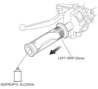
25. Using isopropyl alcohol, remove all traces of adhesive from the left handlebar.
