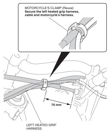
36. Secure the left heated grip harness with the wire tie as shown.
