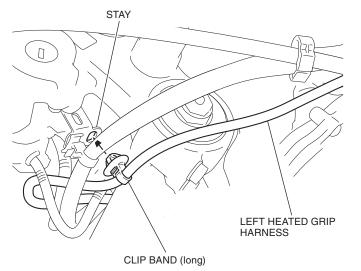
35. Secure the left heated grip harness with the motorcycle's clamp as shown.
