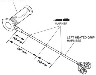
27. Install the clip bands on the marked positions as shown.
