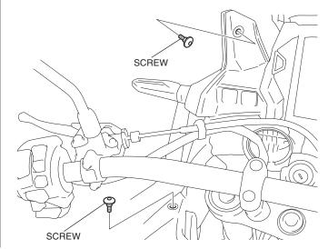
4. Remove the left tank side cover as shown.
