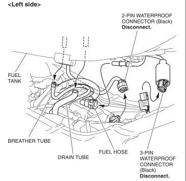
20. Remove the fuel tank as shown.
