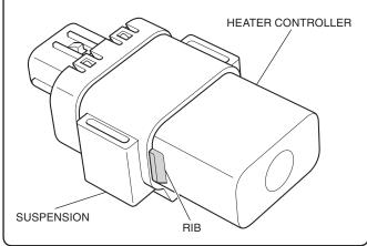
75. Install the heater controller stay as shown.
