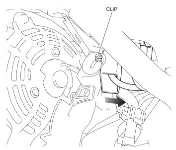
39. Remove the connectors from the stay as shown.
