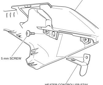
76. Install the heater controller as shown.
