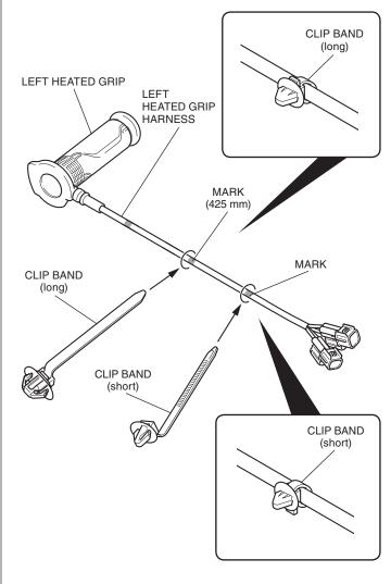
28. Liberally apply the Pro Honda Handgrip Cement to the inside of the left heated grip from kit as shown.
