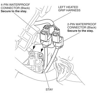
45. Secure the left heated grip harness with the wire tie as shown.
