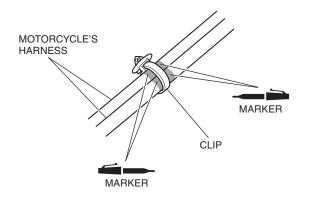
67. Remove the clip from the motorcycle's harnesses as shown.
