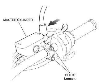
7. Remove the right handlebar switch as shown.
