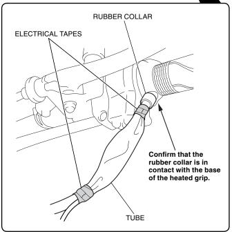
42. Secure each harness with the wire ties as shown.
