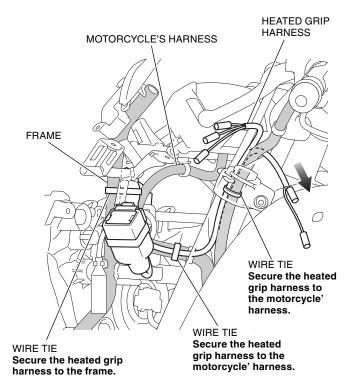
36. Slide the tube over the left heated grip harness as shown.
