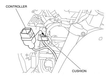
35. Route and secure the heated grip harness with the wire ties as shown.
