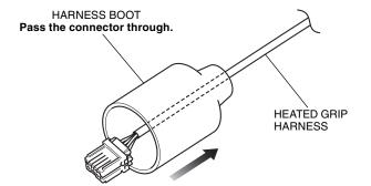
26. Connect the controller as shown.
