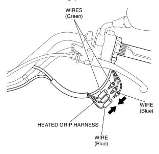
41. Slide and secure the tube with electrical tape as shown.
