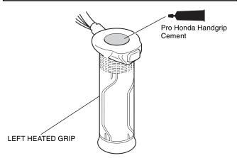
20. Apply Pro Honda Handgrip Cement to the left handlebar as shown.
