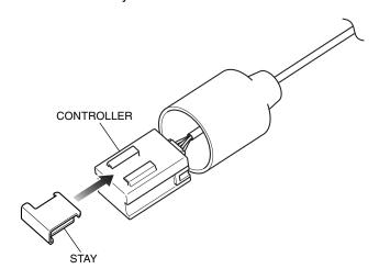
28. Fit the boot over the controller as shown.
