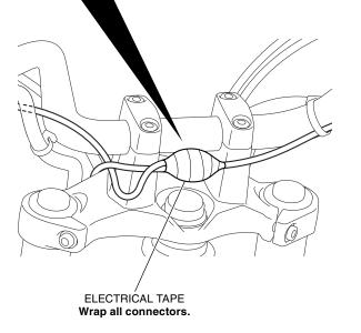
38. Secure each harness with the wire tie as shown.
