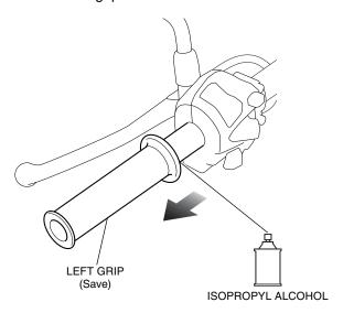
Using isopropyl alcohol, remove all traces of adhesive from the left handlebar.
