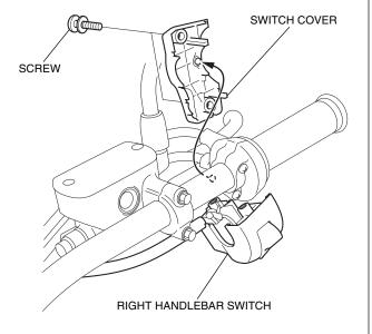
8. Remove the throttle housing cover as shown.
