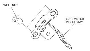
8. Loosely install the left meter visor stay as shown.
