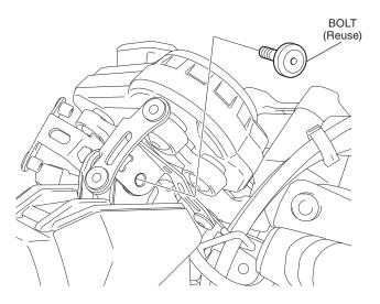
16. Install the meter visor as shown.
