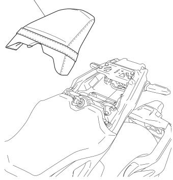
2. Remove the main seat and disconnect the negative (-) cable of the battery.
