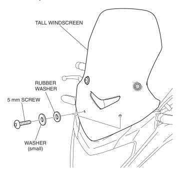
6. Tighten all loosely installed parts securely.
