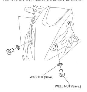
3. Install the well nuts and washers as shown.
