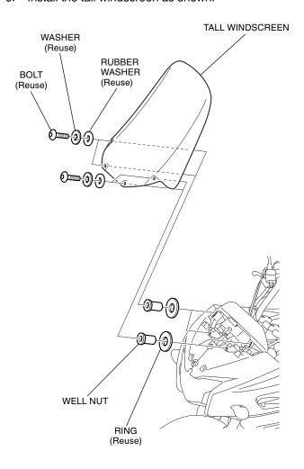
7. Install the motorcycle's parts in the reverse order of removal.
