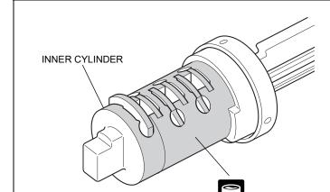
(22)Apply to the tumbler part and to the outer circumference of the inner cylinder.
