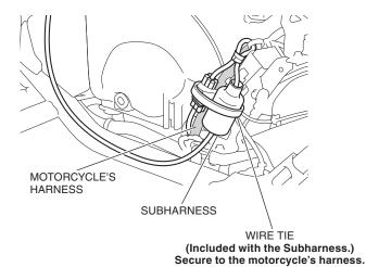
6. Bundle the socket harness and secure it with the wire tie as shown.
