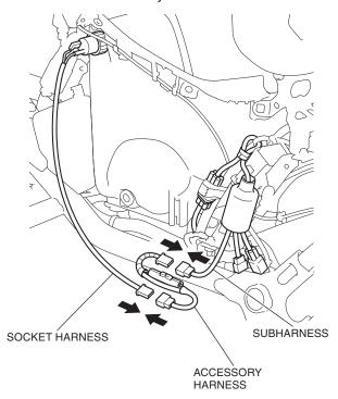
Cover the connectors with the harness boot as shown.
