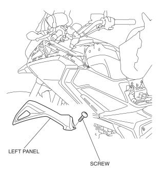
3. Remove the left front side cowl and disconnect the connector.
