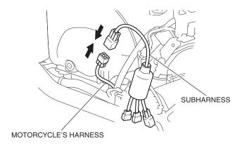
8. Secure the 6-pin waterproof connector with the wire ties and electrical tape as shown.
