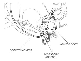
5. Secure the subharness with the wire tie as shown.
