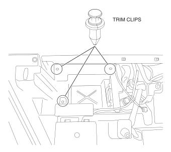
7. Slide the fuse box and mount bracket under the relay fuse box cover and replace the trim clips. Use the remaining trim clips supplied with your mount bracket to secure the two rear mounting points.
