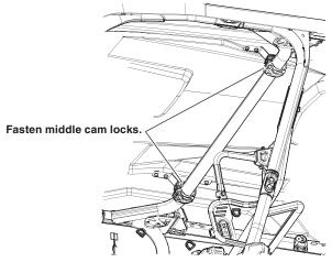
7. Adjust the front cam lock brackets as needed to fit the front OPS bar without the roof bowing or distorting. The cam lock brackets can be adjusted by sliding the bracket along the roof screws as shown.
