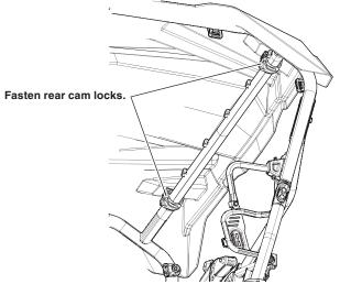
6. Fasten the middle cam locks around the middle OPS bar.
