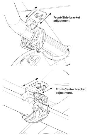
10. The roof should be secure to the touch and should not move once all adjustments are complete.
