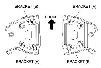
1. Place bracket (B) onto the left A-arm in the position shown.
