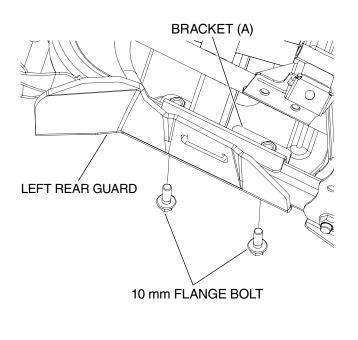
4. Tighten the loosely installed 10 mm flange bolts to the value specified in the Torque Chart.
