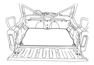
2. Lift the rear seat backs to their upright positions then clip the Carpet Bed Mat "J-Hook" over the seat back cover. Perform step for both seat backs.
