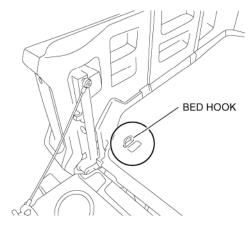
Install the attachment strip through the bed hook then re-secure the strip to the Carpet Bed Mat. Repeat steps 3 and 4 for both sides.
