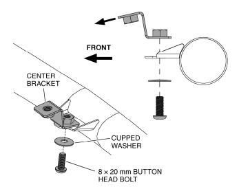
Install the rear mounting bracket to the top of the rear OPS mounting flange using one 8 x 20 mm button head bolt and cupped steel washer.
