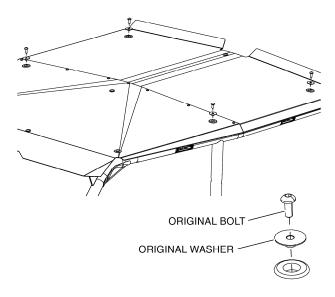
14. Loosely install the roof in the three center locations using three  $8 \times 20$  mm button head bolts and cupped washers as shown.
