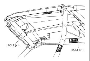
4. Remove the two bolts and spacers securing the original front roof from the outside of the vehicle. Remove the original front roof and set aside.
