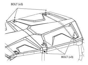
3. Remove the two bolts securing the original front roof on the inside of the vehicle.
