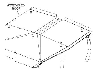
12. Loosely install the roof in the two front corner locations using the original bolts removed in Step 4, as well as one rubber washer and one cupped washer in both locations.
