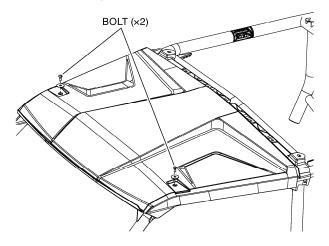
5. Install the front mounting bracket to the top of the front OPS mounting flange using one 8 × 20 mm button head bolt and cupped steel washer. Tighten the hardware securely.
