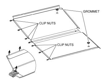
10. Carefully place the rear edge of the front roof over the front edge of the rear roof while lining up the holes in both pieces. Install both roof sections together using seven  $6 \times 16$  mm button head bolts and flat washers as shown. Be sure the hardware is tightened securely.
