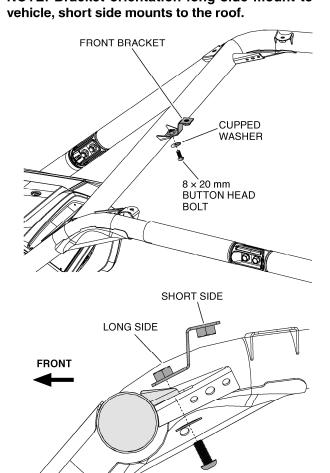
6. Install the center mounting bracket to the top of the center OPS mounting flange using one 8 × 20 mm button head bolt and cupped steel washer. Tighten the hardware securely.
