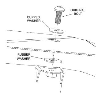
13 Loosely install the roof in the four outside locations with the grommets using the original bolts and washers removed in Step 2.
