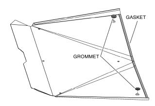
9. Install two rubber grommets and seven clip nuts to the inside of the rear roof as shown.
