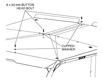
15. Tighten down the fasteners securely in the order shown below to ensure the roof forms around the top of the OPS correctly.
