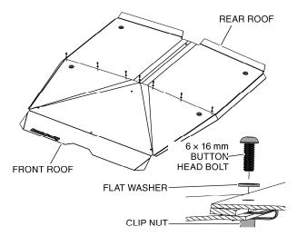
11. Place the roof over the top of the OPS as shown.
