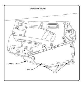
3. Using a center punch or awl, mark the lower door at the center of each crosshair. Carefully remove the template.
