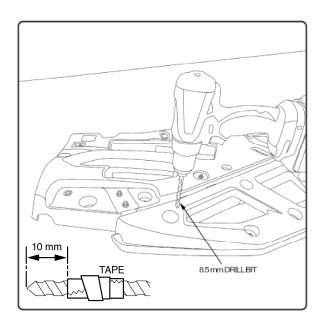
5. Align the holes in the door bag with the drilled holes in the lower door.
