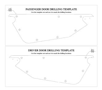
2. Line up the drilling template to the embossed holes on the assembled lower door then tape it in place.
