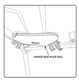
3. Start fastening the outer straps to the cab frame as shown then fasten the straps on the other side.
