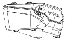
3. Align the rear and front hooks on the corresponding holes of the mounting plate and firmly push the cargo box to engage them. When the hooks are in place, each square hole in the cargo box is also aligned with its corresponding hole in the mounting plate.
