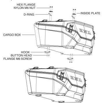
2. Install the left rear hook (9) and the right rear hook (10) with the two inside rear plate (8), two D-ring (11), four M6 button head fl ange screws (12) and four hex fl ange nylon M6 nuts (13). The orientation of the two hooks must be as shown in the pictures below.
