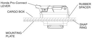
5. Secure the cargo box to the vehicle by pressing down each Honda Pro-Connect lever. Make sure the two hooks and both Honda Pro-Connect latches are well engaged.
