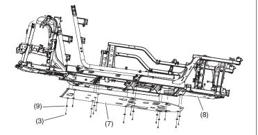
5. Install the 6 x 40 mm socket bolts in the remaining hole of the aluminum spacer. Install the 6 x 12 mm socket bolts at the front area of the main skid plate.
