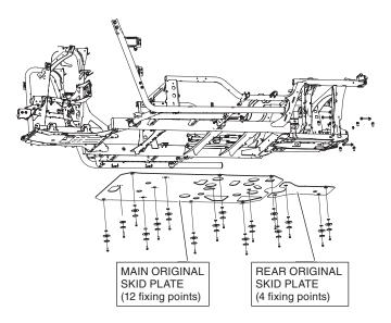
2. Install the new rear skid plate. Loosely tightened the two 6 x 16 mm flat head socket bolt and washers.
