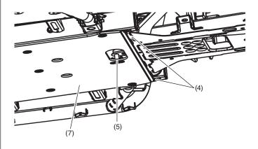
6. Adjust and position both skid plates and secure every fastener to the required torque from chart on first page.
