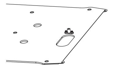
4. Install the new main skid plate. Align new main skid plate to the holes in the rear skid plate. Loosely tighten all fasteners (flat head socket bolt  $6 \times 16 \, \text{mm}$  and washer).
