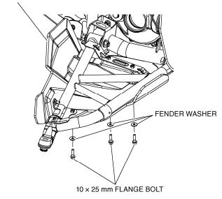
5. Tighten all the bolts the value specified in the TORQUE CHART starting with the one facing forward.
