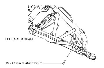
4. Loosely install the fender washers and the 10  $\times$  25 mm flange bolts starting with the closest to the wheel.
