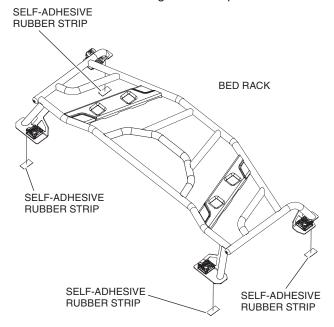
4. Make sure the Honda Pro-Connect latch levers are in the open position then locate the Bed Rack onto the Vehicle Bed by aligning each Honda Pro-Connect latch with his corresponding bed installation hole. Lock the Bed Rack in place by pressing down the four Honda Pro-Connect latch levers. To remove the Bed Rack from the vehicle, just lift the lever from each Honda Pro-Connect latch and freely remove the accessory.
