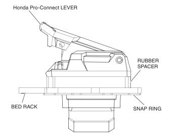
Remove the film from the self-adhesive rubber strips and stick them to the Bed Rack in the position shown in the view below.
