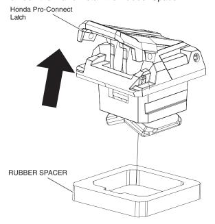
Insert the assembled Honda Pro-Connect latch with the rubber spacers in the Bed Rack installation square holes and secure them by using the Snap Rings.
