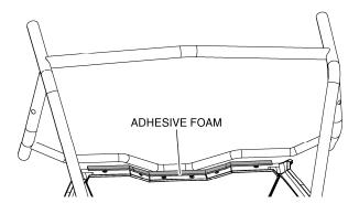
5. Install the flocked trim into the channel along the top edge of the lower mounting bracket as shown.
