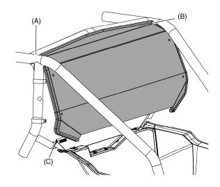
9. Adjust the position of the rear panel as needed to line up the mounting holes in the rear panel with the clamps. Make sure the lower edge of the rear panel is inside of the channel on the mounting bracket.
