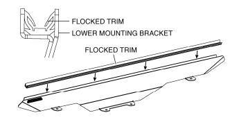
6. Place the lower mounting bracket just behind the horizontal OPS tube behind the seat. The mounting flange in the center of the lower mounting bracket will rest on top of the seat back upper cover. The "HONDA" logo can be seen from the outside of the vehicle.
