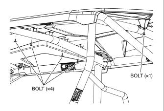
2. Remove the six bolts securing the original rear roof from the outside of the vehicle. Remove the original rear roof and set aside.
