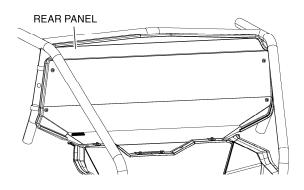
10. Loosely attach all four clamps to the rear panel using one 25 mm hex head bolt, shoulder spacer, and 6 mm Nylock flange nut per clamp. Once all four clamps have been attached to the rear panel, tighten the hardware until the first three threads on each screw are visible outside of the nut.
