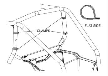
8. Lift the rear panel into place so the mounting hole in the driver's side corner of the rear panel (A) is near the upper clamp on the vertical OPS tube. Repeat on the passenger side (B), then lower the bottom edge down into the channel on the mounting bracket (C).
