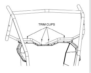
4. Remove the backing from the adhesive foam and apply it along the base of the body panel just above the trim clips removed in the previous step.
