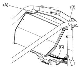
Adjust the position of the rear panel as needed to line up the mounting holes in the rear panel with the large and small clamps. Make sure the lower edge of the rear panel is inside of the channel on the mounting bracket.
