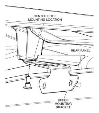
16. From inside of the vehicle, loosely attach the upper mounting bracket to the rear panel using two shoulder spacers and 6 mm Nylock nuts as shown.
