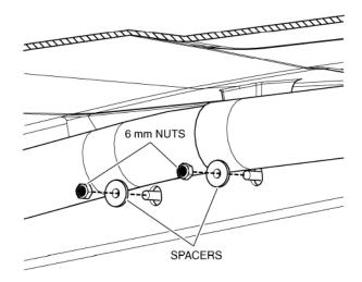
17. Adjust the position of the rear panel, lower mounting bracket, and clamps as needed, then tighten all hardware securely.
