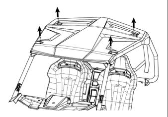
2. Remove the two original bolts securing the roof from the inside of the vehicle. Remove the roof and set aside.
