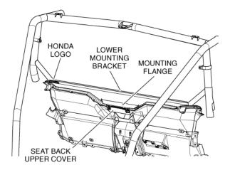
8. Lift the rear panel into place so the mounting hole in the driver's side corner of the rear panel (A) is near the large clamp on the vertical OPS tube. Repeat on the passenger side (B), then lower the bottom edge down into the channel on the mounting bracket (C) as shown.
