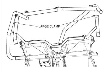
7. Place the lower mounting bracket just behind the horizontal OPS tube behind the seat. The mounting flange in the center of the lower mounting bracket will rest on top of the seat back upper cover. The HONDA logo can be seen from the outside of the vehicle.
