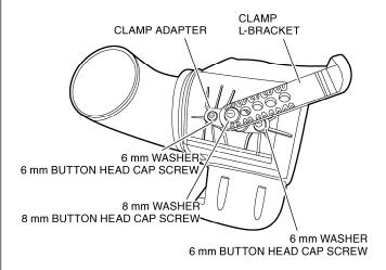
15. Attach the clamp L-bracket to the clamp pivot using the 8 mm washer and the  $8 \times 22$  mm button head cap screw. Do this for both sides and hand tighten to verify desired position. Once position is verified, tighten the straps securely to the bars.
