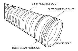
18. Place the hose clamp size #56 onto the flex duct end cuff clamp groove and slide everything over the upper tube until the flex duct end cuff reaches the bead on the upper tube as shown. Tighten the hose clamp.
