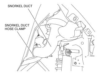
5. Remove the three trim clips from snorkel duct then remove the snorkel duct.
