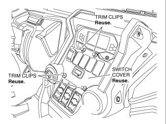
33. Reinstall the upper center console removed in Step 24. Make sure to insert the prong into the grommet.
