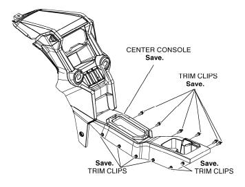
24. Remove the upper center console between the seats by pulling it towards the front of the vehicle and releasing the prong from the grommet.
