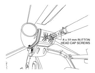
17. Carefully slide the flex duct end cuff over the 3.5 in ID flexible duct until the end of the duct reaches the inside bead of the flex duct end cuff as shown.
