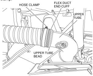
19. Position the flexible duct on the particle separator in the desired position and mark the ducting 2" past the particle separator outlet.
