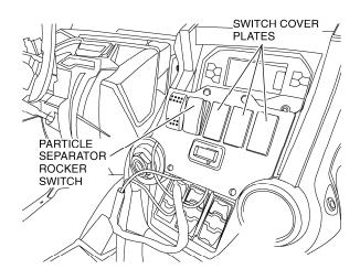
27. Remove hood and four trim clips holding the rubber mud guard and move it out of the way to access the back side of the switch panel compartment.
