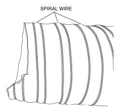
21. Carefully slide the flex duct end cuff over the 3.5 in ID flexible duct until the end of the duct reaches the inside bead of the flex duct end cuff as shown.
