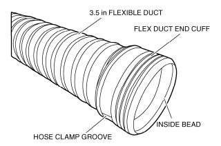
22. Place the hose clamp size #56 onto the flex duct end cuff clamp groove until the flex duct end cuff covers at least 2 in of the particle separator outlet as shown. Tighten the hose clamp.
