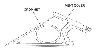
9. Install the vent cover to the vehicle and secure it using four trim clips removed in Step 1.
