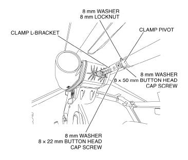
16. Support the Particle Separator Unit then add a drop of Threadlocker to the ends of the four  $8 \times 22$  mm Button Head Cap Screws, one at a time, previously installed in Steps 12 and 13.
