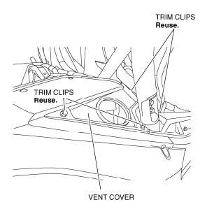
10. Install the upper tube into the vent cover through the grommet as shown.
