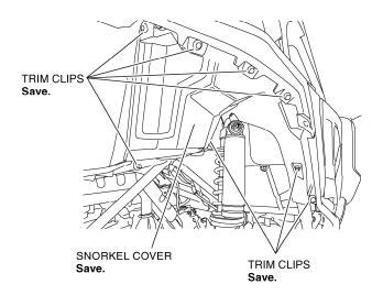
3. Remove the two trim clips from the right rear over fender and remove them. Remove the snorkel cover from the vehicle.
