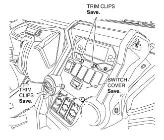
26. Remove a desired switch cover plate then place the particle separator rocker switch into the open space.
