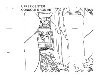
25. Remove the four trim clips that hold the switch cover then remove the switch cover.
