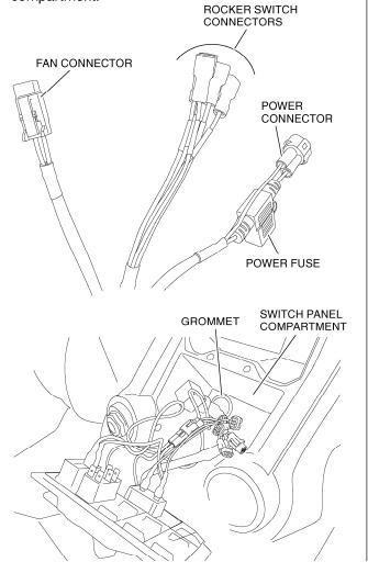
29. Route the fan connector from the grommet back through the center console area and up along side the OPS to the fan on the particle separator. Connect the wire harness fan connector to the particle separator fan connector. Use cable ties to secure the harness in several locations along side the main harness as shown in the illustrations.
