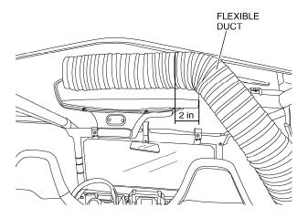
20. Using a utility knife, cut the flexible duct at the mark keeping the blade between the spiral wires then use wire cutters to cut the wire at the end as shown.
