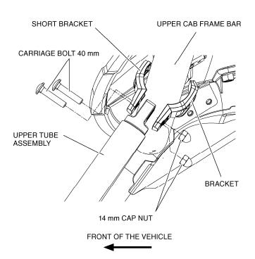
3. Loosely install the right side of the lower tube with the brackets, carriage bolts 40 mm and 14 mm cap nuts. Repeat on the left side.
