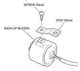
12. Install the suspension on the back-up buzzer as shown.
