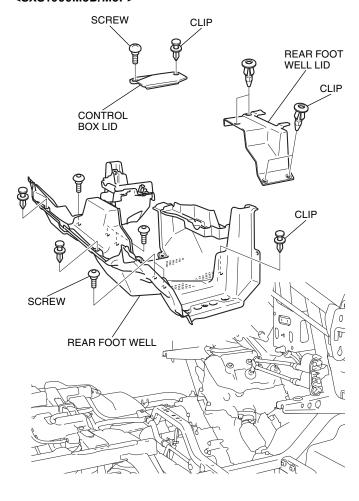
11. Remove the parts as shown.
