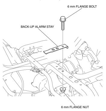
14. Install the assembled back-up buzzer on the back-up alarm stay.
