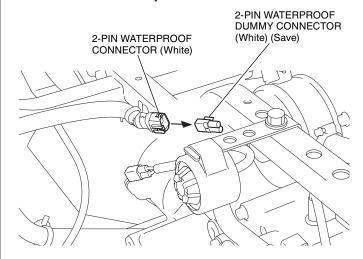
16. Connect the back-up buzzer harness as shown.
