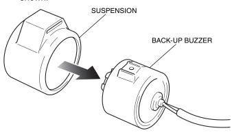
13. Install the back-up alarm stay as shown.
