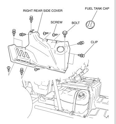
6. Install the fuel tank cap as shown.
