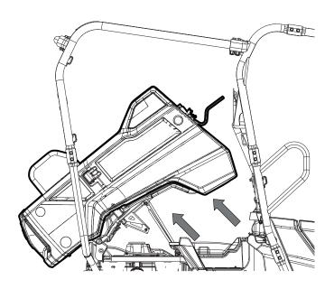
2. Refer to Service Manual to remove the center rear foot well (M4/M4D types only).
