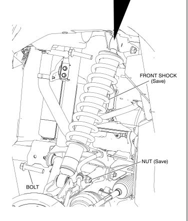
3. Install the accessory shock absorber as shown.
