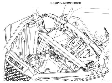
7. Connect the accessory sub-harness to the DLC (4P Red) connector.
