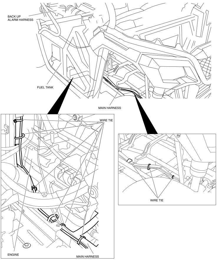
5. Follow the main harness going up. Secure the back up alarm harness to the main harness with wire ties along the front right side of the vehicle as shown.
