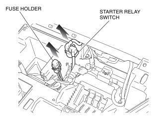
15. Remove the connectors as shown.
