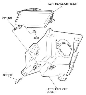
24. Install the headlight caps on the left LED headlight as shown.
