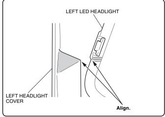
26. Install the assembled left headlight cover in the reverse order of removal.
