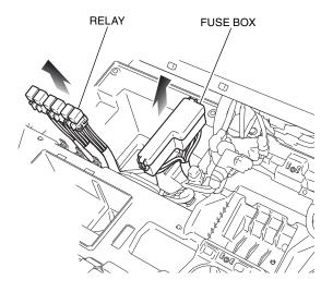
14. Remove the fuse holder and starter relay switch as shown.
