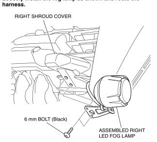
61. Connect the fog lamp sub harness to the right LED fog lamp harness as shown.
