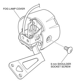
51. Route the left LED fog lamp harness and install the fog lamp cap as shown.
