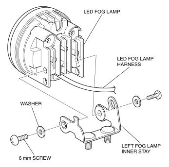
45. Install the 6 mm nut to the LED fog lamp as shown.
