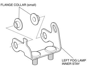
44. Loosely install the assembled left fog lamp inner stay as shown.
