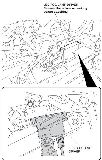
33. Remove the dummy connector as shown.<Right side>
