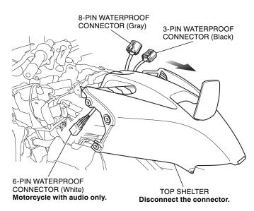
19. Raise the front side of the top shelter and remove the right panel switch as shown.
