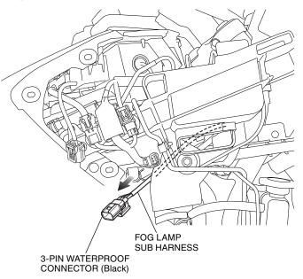
39. Remove the dummy connector as shown.
