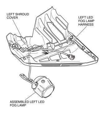
55. Secure the left LED fog lamp harness as shown.
