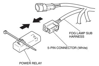
29. Secure the power relay as shown.
