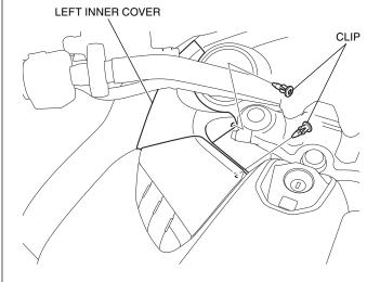
2. Remove the left inner cover, and disconnect the negative (-) cable of the battery.
