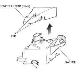
22. Install the fog lamp switch knob as shown.
