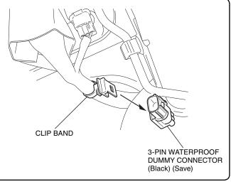
40. Secure the connector as shown.
