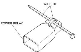
28. Connect the power relay as shown.
