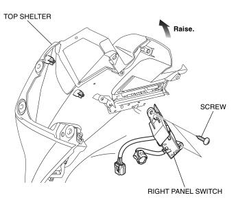
20. Remove the switch as shown.
