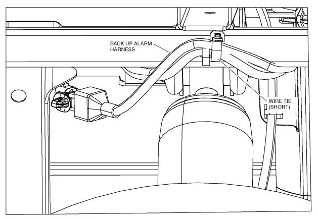
5. Continue securing the back up alarm harness. Follow the main harness down near the back of the engine, under the passenger seat as shown, and secure the back up alarm harness to the main harness with wire ties.
