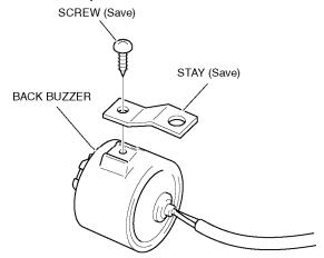
10. Install the suspension on the back up buzzer as shown.
