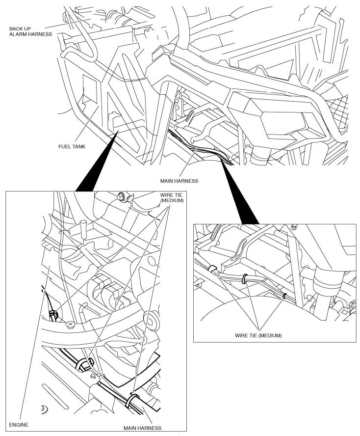
6. Follow the main harness going up. Secure the back up alarm harness to the main harness with wire ties along the front right side of the vehicle as shown.
