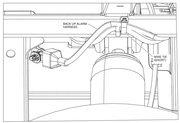
5. Continue securing the back up alarm harness. Follow the main harness down near the back of the engine, under the passenger seat as shown, and secure the back up alarm harness to the main harness with wire ties.
