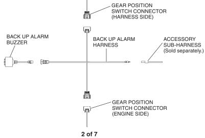
4. Follow the main harness toward the rear of the vehicle. Secure the back up alarm harness to the main harness with wire ties in the locations shown.
