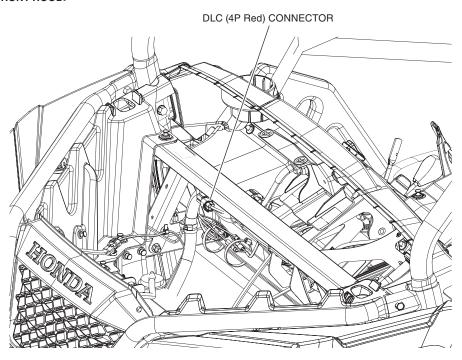
8. Connect the accessory sub-harness to the DLC (4P Red) connector.
