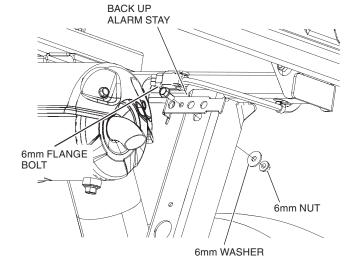
12. Install the assembled back up buzzer on the back up alarm stay.
