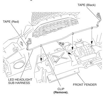
34. TRAIL and FOREST models only. Use supplied clips to band the headlight sub harness to the winch harness and install clips to the fender as shown.
