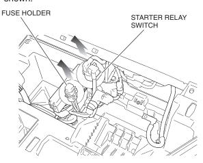
15. Remove the connectors as shown.
