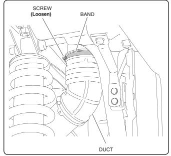
2. Remove the vehicle's parts as shown.
