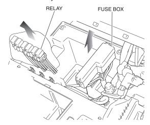
14. Remove the fuse holder and starter relay switch as shown.
