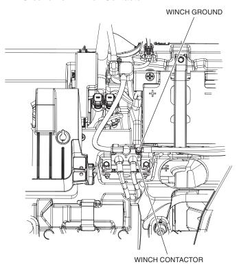
18. TRAIL and FOREST models only. Remove Battery+ connection from winch contactor.
