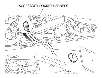
29. Remove the dummy connector from the 2P black connector shown.
