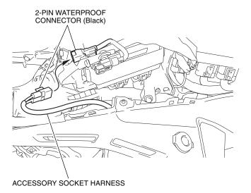
31. Secure the accessory socket harness with the wire ties as shown.
