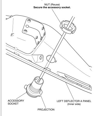
28. Route the accessory socket harness as shown, and install the left deflector panel A and parking lever in the reverse order of removal.
