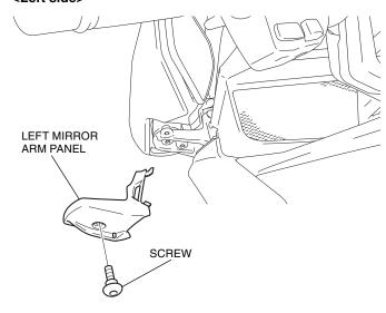
7. Remove the left rear view mirror as shown.
