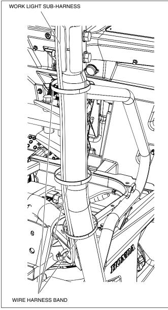
17. Continue to route the Work Light Sub-Harness along the cab frame B-pillar and secure it with wire harness bands in the positions shown.
