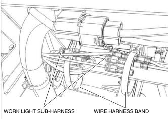
12. Route the Work Light Sub-Harness alongside the vehicle Main Wire Harness and secure it with wire harness bands in the positions shown.
