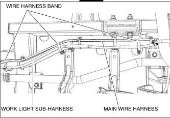
14. Continue to route the Work Light Sub-Harness alongside the vehicle Main Wire Harness and secure it with wire harness bands in the positions shown..
