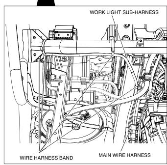
16. Continue to route the Work Light Sub-Harness along the cab frame B-pillar and secure it with wire harness bands in the positions shown.
