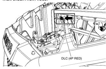
6. Connect the Accessory Sub-Harness to the DLC (4P Red) connector as shown.
