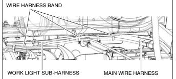
15. Continue to route the Work Light Sub-Harness alongside the vehicle Main Wire Harness and secure it with wire harness bands in the positions shown.
