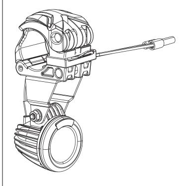
4. Install the Work Light assembly to the rear cab frame cross member as shown.
