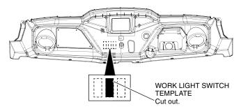
9. Install the Work Light Switch into the cut-out in the instrument panel as shown.
