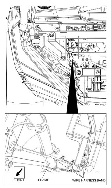
13. Continue to route the Work Light Sub-Harness alongside the vehicle Main Wire Harness and secure it with wire harness bands in the positions shown.
