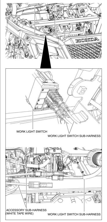
11. Route the Work Light Sub-Harness as shown and secure it with wire harness bands in the positions shown.
