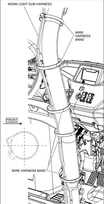
18. Continue to route the Work Light Sub-Harness along the cab frame rear cross member and secure it with wire harness bands in the positions shown. Connect the Work Light Sub-Harness to the Work
